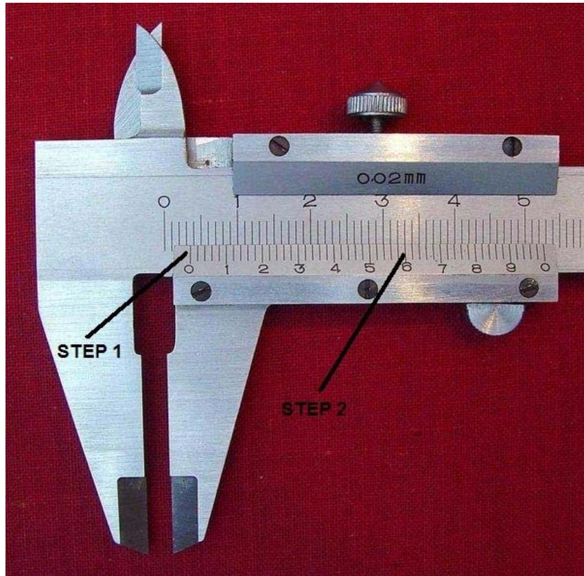
Figure 2.3.5: Reading Vernier Scales
