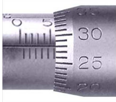
Figure 2.3.14: Metric Micrometer Scales
