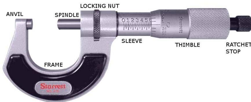
Figure 2.3.10: Outside Inch Vernier Micrometer
