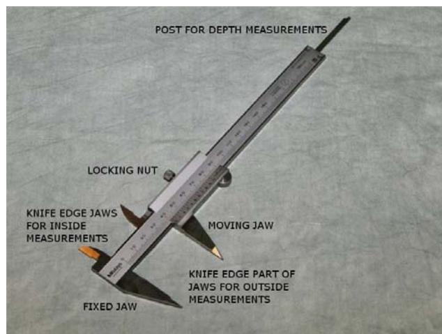
Figure 2.3.4: Components of a Vernier Caliper
