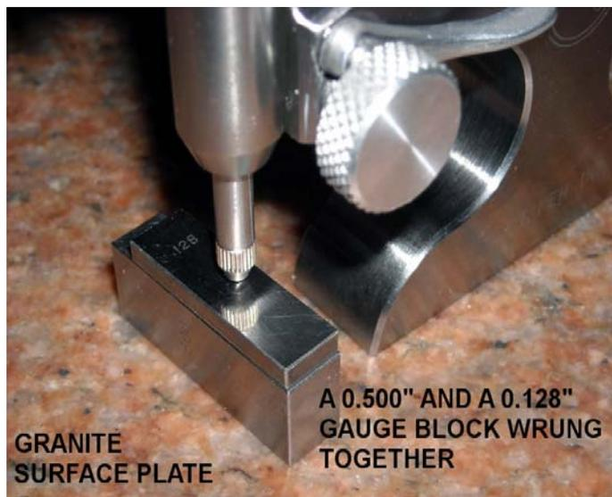
Figure 24.8: Wrung Gauge Blocks
