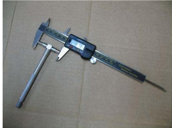
Figure 2.4.3: Telescoping Gauge and Vernier Caliper
