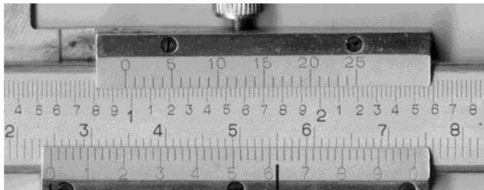
Figure 2.3.7: Dual Vernier Scales
