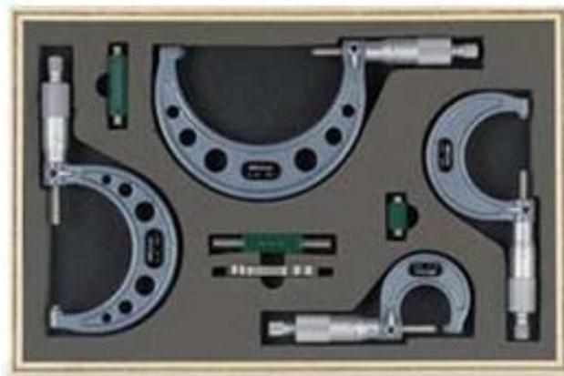
Figure 2.3.11: Micrometer Set 1" to 4"
