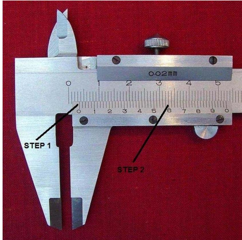
Figure 2.3.5: Reading Vernier Scales
