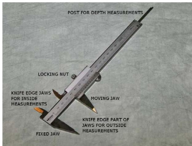
Figure 2.3.4: Components of a Vernier Caliper
