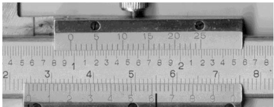
Figure 2.3.7: Dual Vernier Scales
