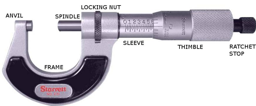
Figure 2.3.10: Outside Inch Vernier Micrometer
