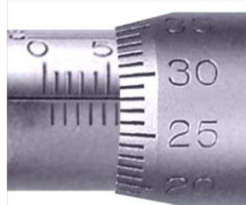
Figure 2.3.14: Metric Micrometer Scales
