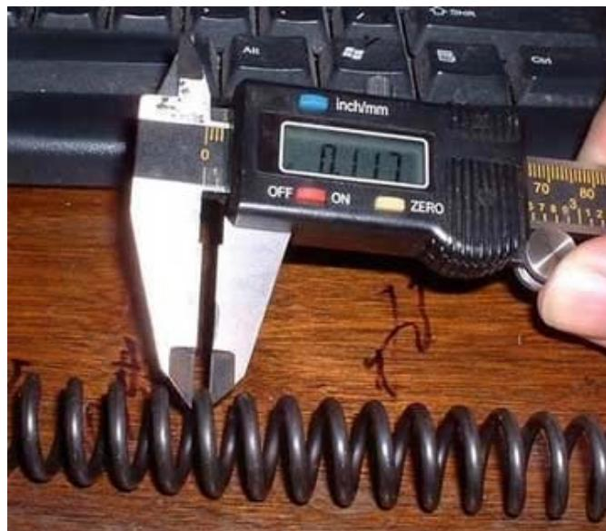
Figure 2.3.9: Digital Caliper
