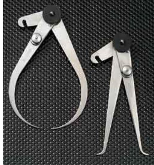
Figure 2.4.1: Transfer Calipers
