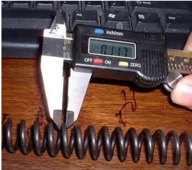
Figure 2.3.9: Digital Caliper
