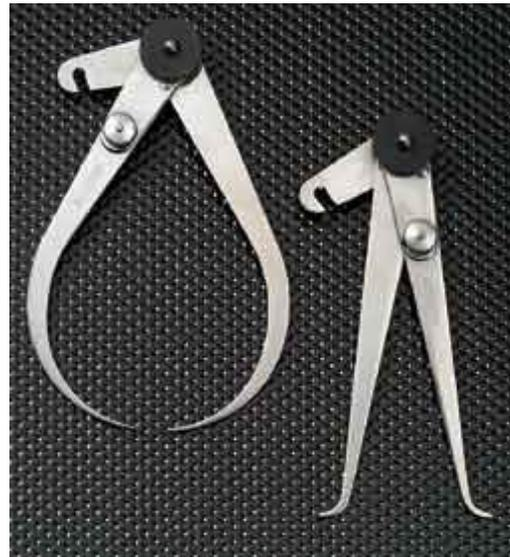
Figure 2.4.1: Transfer Calipers
