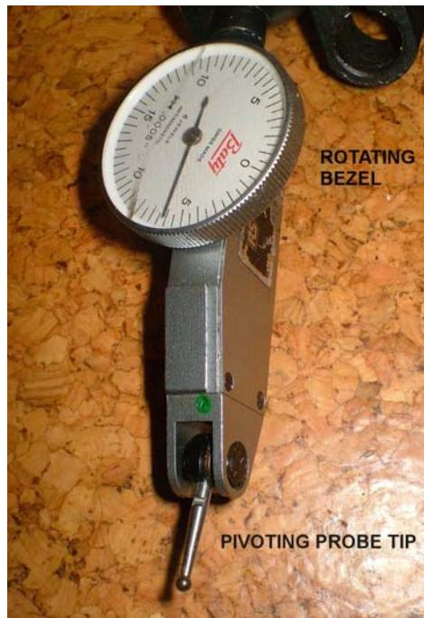
Figure 2.4.6: Dial Test Indicator
