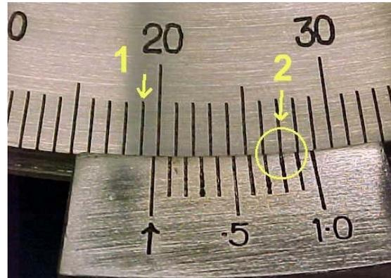
Figure 2.3.6: Angular Vernier Scale
