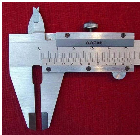
Figure 2.3.2: Metric Vernier Caliper
