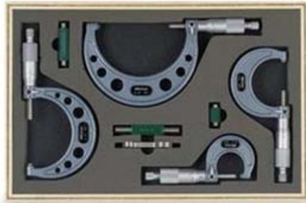
Figure 2.3.11: Micrometer Set 1" to 4"
