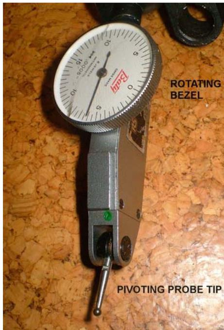
Figure 2.4.6: Dial Test Indicator
