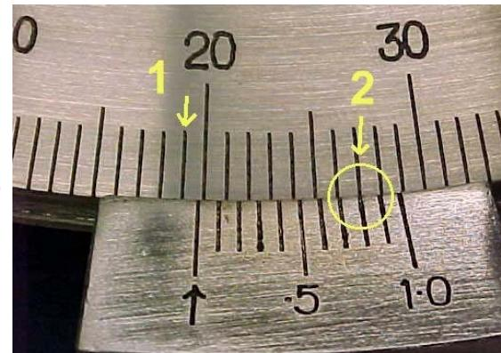
Figure 2.3.6: Angular Vernier Scale
