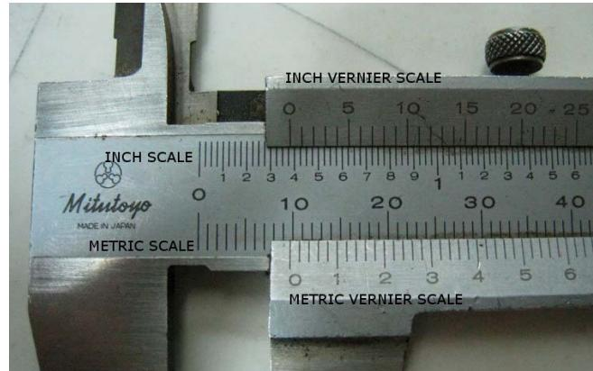
Figure 2.3.3: Dual Unit Vernier Caliper
