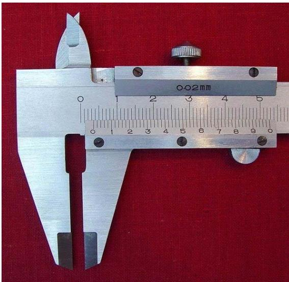
Figure 2.3.2: Metric Vernier Caliper
