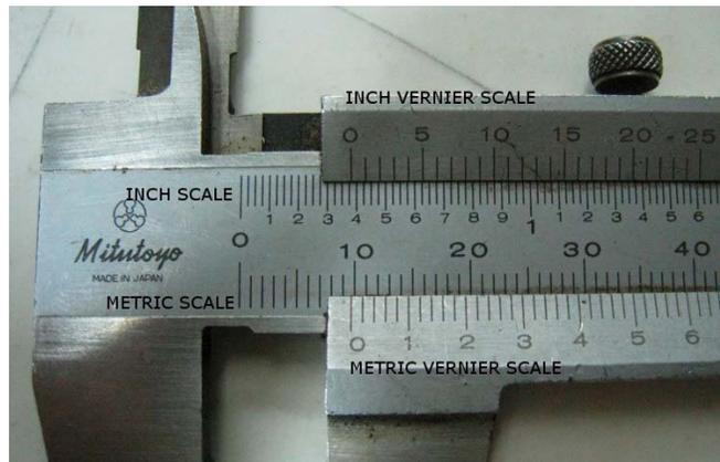
Figure 2.3.3: Dual Unit Vernier Caliper
