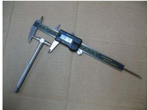
Figure 2.4.3: Telescoping Gauge and Vernier Caliper
