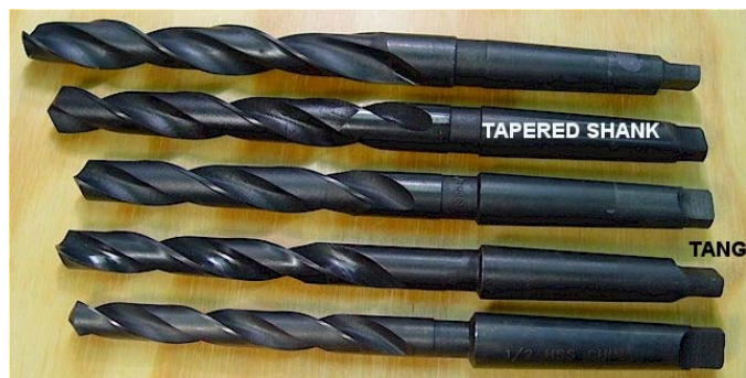
Figure 1.1.10: Tapered Shank with Tang Drill Bits \frac{1}{2} " to \frac{3}{4} "
