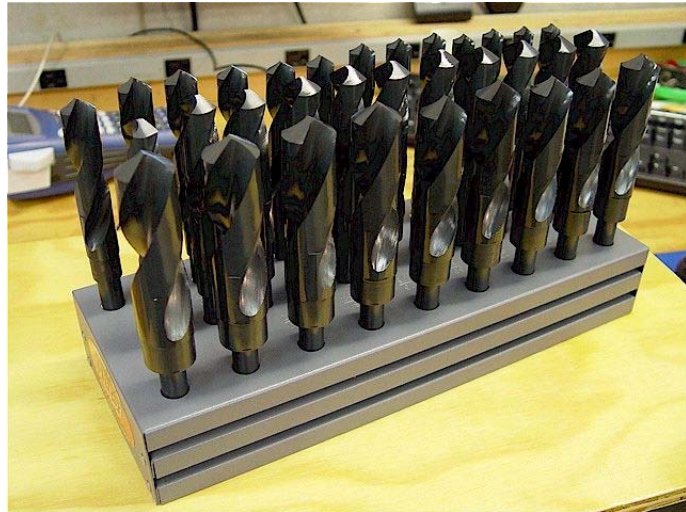
Figure 1.1.9: \frac{1}{2} " to 1" Bits with \frac{1}{2} " Shank
