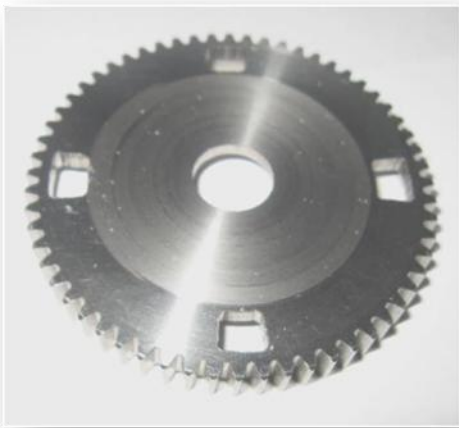
Fig.9.2 Machined Top Clutch Plate
