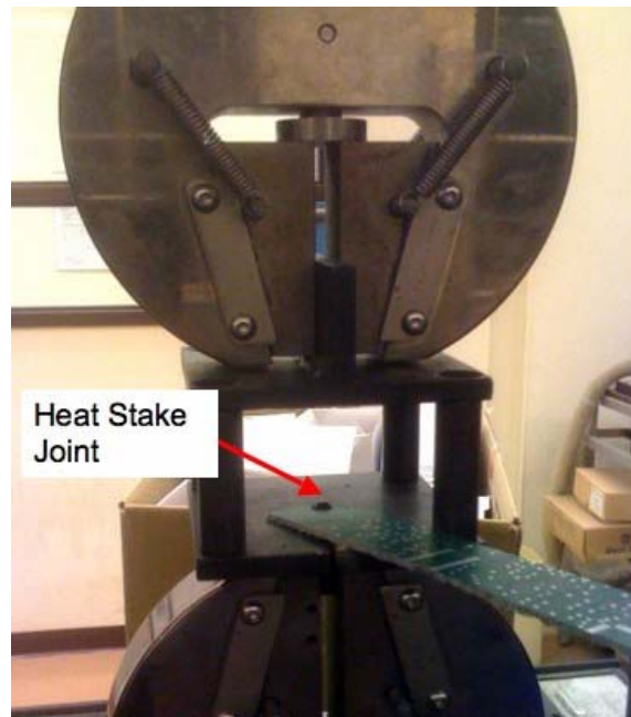
Figure 2-18 Heat stake sample testing in Instron Machine
