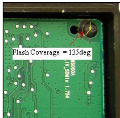
Figure 2-9 Measurement of flash on heat stake head
