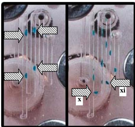
Figure 10. Liquid water collection interior land test; left (a): before, right (b): after. Arrows indicate areas with liquid mentioned in the report.
