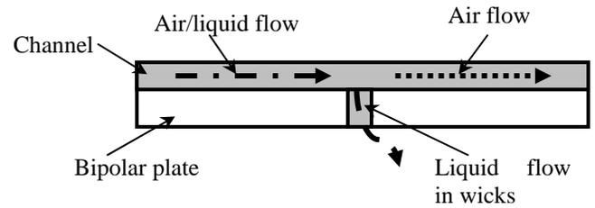
**Figure 2. Liquid water collection concept – channel well idea.**
