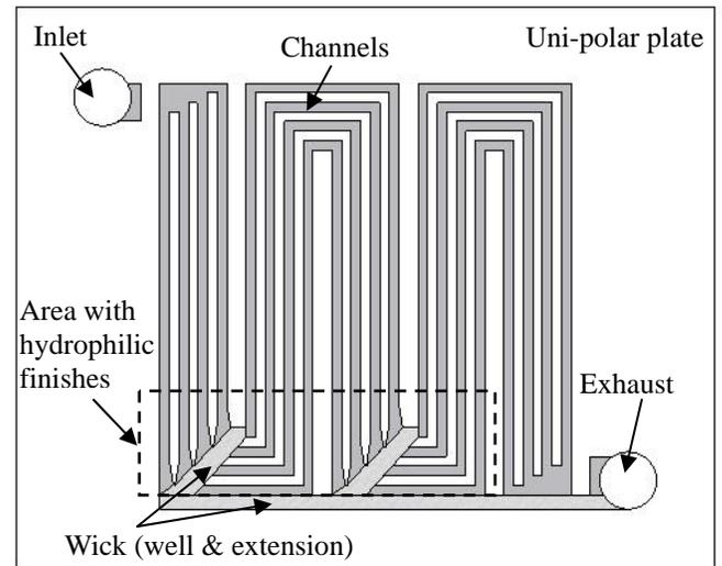
**Figure 14. A possible implementation for the liquid water removal concept.**
