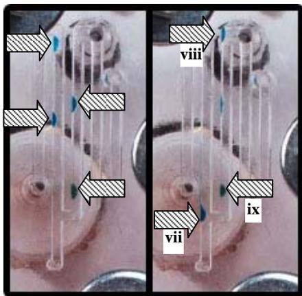
Figure 9. Liquid water collection exterior corner test; left (a): before, right (b): after. Arrows indicate areas with liquid mentioned in the report.
