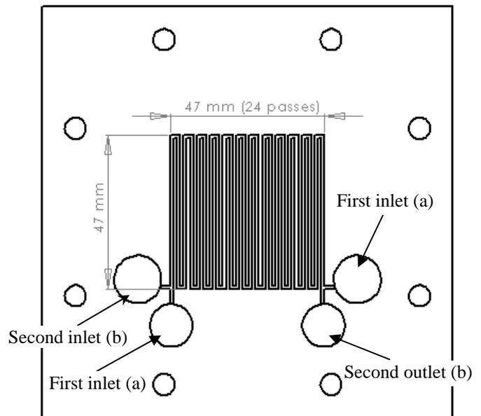
**Figure 4. A 1.1m serpentine flow field for the flow direction reversal apparatus.**
