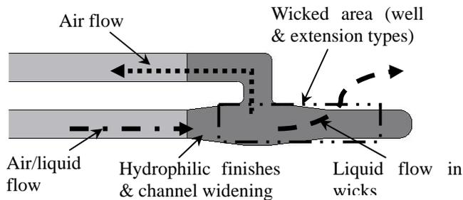
**Figure 12. Enhanced liquid water collection concept.**
