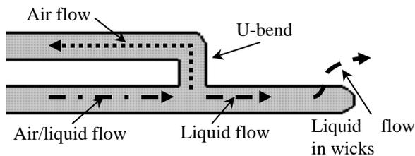
**Figure 1. Liquid water collection concept – channel extension idea.**
