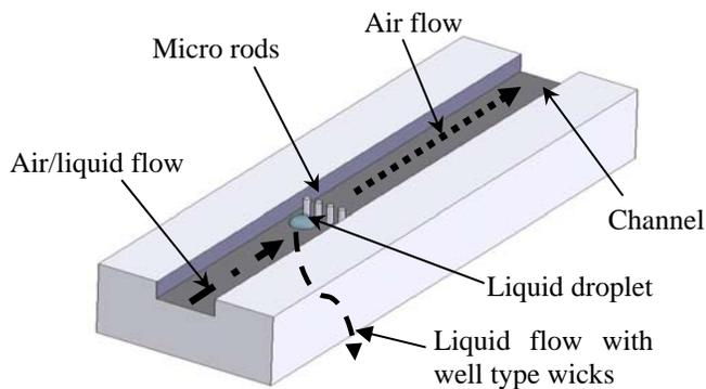
**Figure 13. Trapping liquid with hair-like features.**
