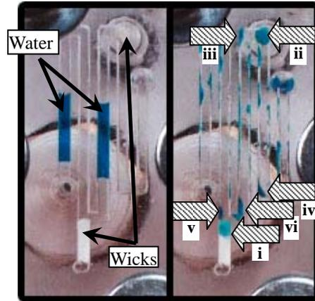
**Figure 8. Liquid water collection test; left (a): before, right (b): after. Arrows indicate areas with liquid mentioned in the report.**
