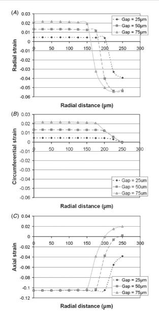
**Figure 4.** Simulated effect of a gap size between the loading piston and the compression chamber side wall on strain distribution within semi-confined cylindrical hydrogel constructs for (A) radial, (B) circumferential, and (C) axial strains. Error bars have been omitted for clarity, but follow similar patterns as in figure 3(C). Standard deviations reduce in magnitude with decreasing gap size in the central region of the hydrogel under uniform strain.
