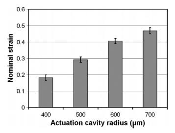
**Figure 5.** Experimental characterization of PEG hydrogel deformation for an applied pressure of 55 kPa across the microdevice array. Increasing actuation cavity size increases strains applied to the cylindrical microconstructs. Nominal strain values reported are for the deformation of the loading piston into the biomaterial, and error bars represent the standard deviation in measurement for a single microconstruct (n = 3).
