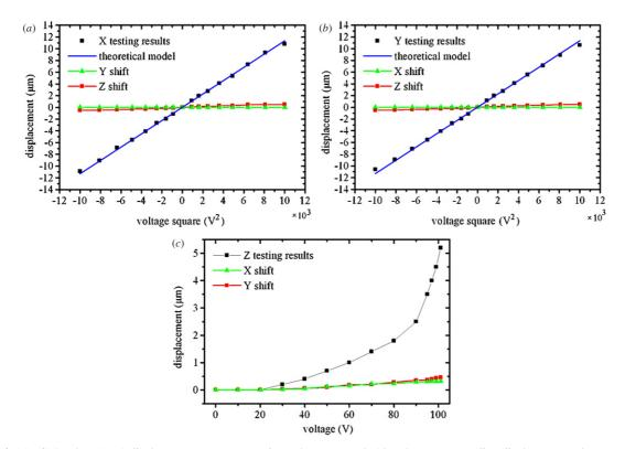
Figure 6. (*a*), (*b*) In-plane (x-y) displacements versus actuation voltage squared. Also shown are coupling displacements along un-actuated directions. (*c*) Out-of-plane displacements before pull-in versus actuation voltages.
