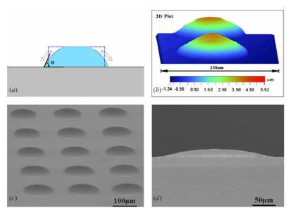
**Figure 3.** (*a*) Schematic of PDMS pre-polymer reflow. (*b*) 3D optical profilometer measurement of PDMS microlenses. Partial curing time: 0 s,  $\alpha = 7.9^{\circ}$ . (*c*) SEM picture of a microlens array. (*d*) SEM picture of the cross section of a PDMS microlens. Partial curing time: 10 s,  $\alpha = 22.5^{\circ}$ .
