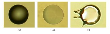
Figure 2. Optical microscopy pictures of patterned PDMS membranes with 50  $\mu$ m bottom diameter under different partial curing times. (a) 10 s, (b) 25 s, (c) 40 s.
