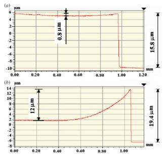
**Figure 4.** Optical profilometer measurement results of PDMS membrane top surfaces. (*a*) PDMS membrane produced using parylene C lift-off. (*b*) PDMS membrane produced using blade scratching.
