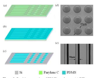
**Figure 1.** Precision patterning of PDMS membranes. (*a*) RIE pattern LPCVD parylene C. (*b*) PDMS spin coating. (*c*) Peeling away parylene C. (*d*), (*e*) Patterned PDMS membrane examples (15  $\mu$ m thickness).
