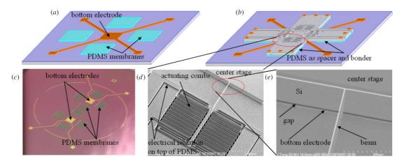
**Figure 5.** A 3-axis positioning stage with patterned PDMS membranes used as a bonding material and as a precisely defined spacer. (*a*) Lift-off patterning of Au/Cr and PDMS membrane patterning according to figure 1. (*b*) DRIE etch top thin silicon wafer to form suspended structures. (*c*) Device picture of PDMS membranes and bottom electrodes. (*d*) A completed device 3-axis positioning stage. (*e*) A 15  $\mu$ m gap between stage and substrate.
