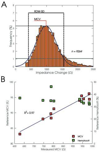
**Fig. 6** RBC measurement results. (A) RBC size histogram highlighting measured RBC indices: distribution width (RDW-SD) and mean corpuscular volume (MCV). (B) Correlation plot for mean corpuscular volume (MCV): reference hematology analyzer (*y*) *vs.* microfluidically measured MCV (*x*). Line fitting generates a correlation coefficient of 0.97.
