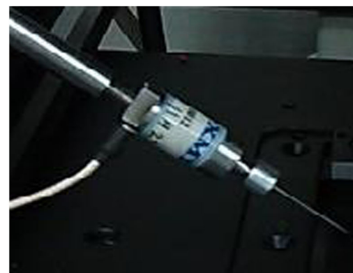
Fig. 1 a System setup for micro-dissection of thin tissue sections b Stack piezoelectric actuator
