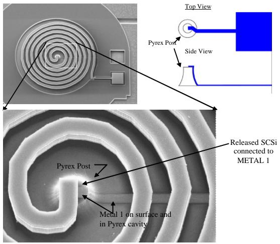
Figure 3-5 – Inductor example to show Metal 1 to Metal 2 connection through the silicon and Metal 1 on the surface of the Pyrex.
