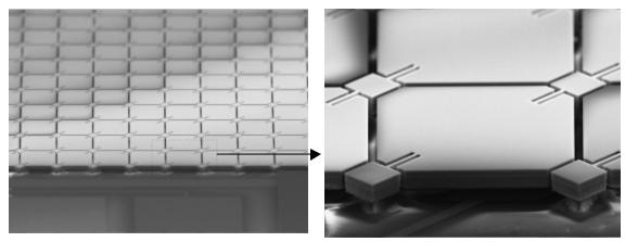
Example 4: Optical MEMS - Digital Mirror Array
