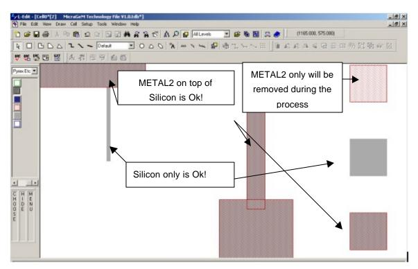
Figure 3-9: METAL2 Features Must Appear on Top of SCSi Layer
