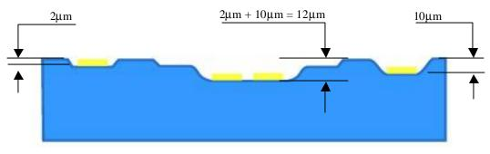
Figure 3-1: Multi Pyrex Cavity Depths
