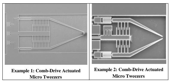
Figure 6-1: Comb-Drive Actuated Micro Tweezers
