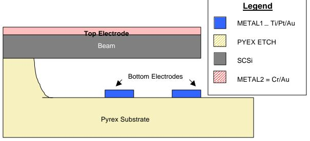
Figure 2-1: Side View of Cantilever Beam Designed with Micragem
