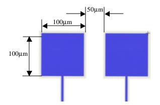
Figure 5-1: Minimum Bonding Pad size and Pitch
