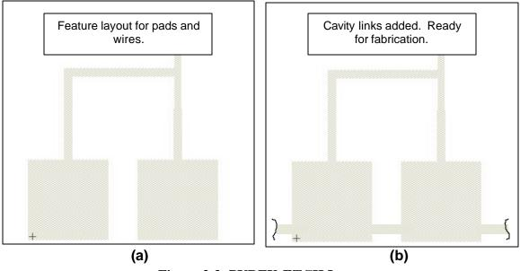
Figure 3-3: PYREX ETCH Layer
