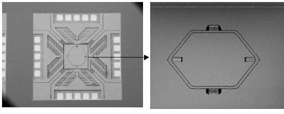
Example 3: Optical MEMS - 3D Optical Mirror
