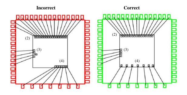
**Figure 5-2: Bonding Requirements Illustrated**
