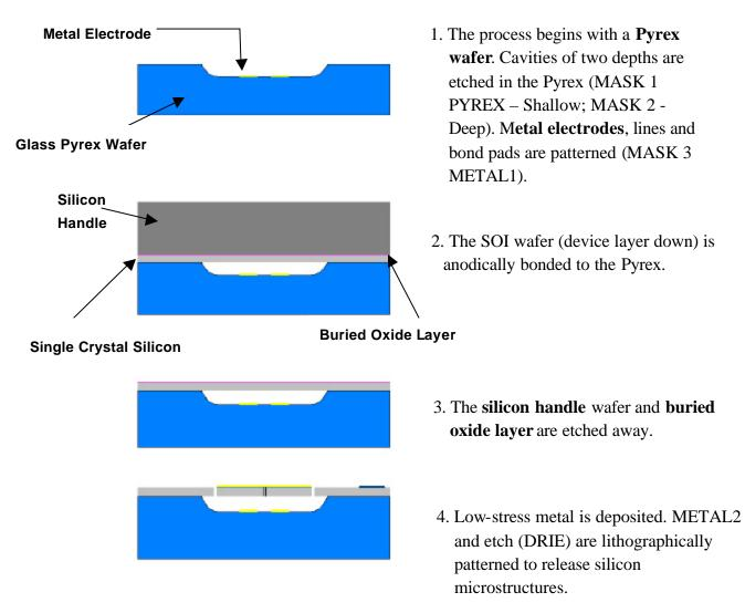
Figure 1-1: Steps in the Micragem Prototyping Process
