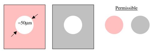
Figure 3-10: Etched circles less than 50mm not allowed in Metal 2 and SCSi Layers
