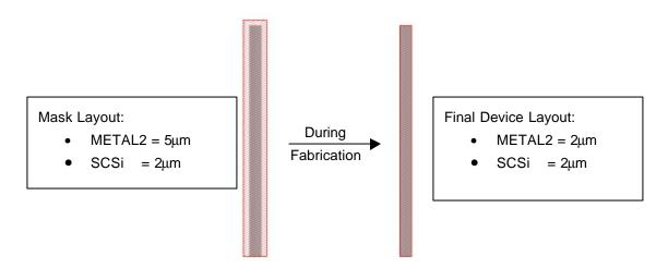
Figure 3-7: METAL2 Self Aligned to Released Silicon Features
